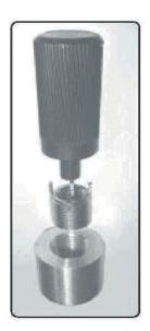
One-piece Keensert inserts are supplied with kees pre-assembled into dove-tailed slots for ease of installation. The pre-positioned kees automatically set the insert to the correct depth below the material surface. Unlike conventional inserts, there is no need to maintain critical depth tolerances and no chance of inadequate locking or deformation of internal threads due to miss calculations of depth. For critical edge distance applications, please consult your Sales Engineer.
