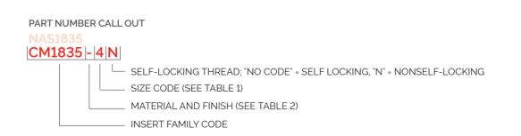
PART NUMBER CALL OUT: CM1835-CARBON STEEL-CADMIUM PLATE-.3750-24-NONSELF-LOCKING
