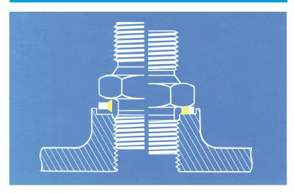
The bonded seal was originally designed to replace copper type washers in higher pressure systems. Simple in construction the gasket comprises a metal annulus, square or rectangular in section, to which an elastomeric ring of trapezoidal section is bonded. The metal ring resists the bursting forces and limits the deformation of the elastomeric element.
