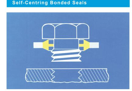
Developed to eliminate the occurrance of leakage due to seal offset, the centring type of bonded seal has the additional benefit of pre-assembling on to threads with the consequent production line savings. The thin seal membrane offers little resistance during assembly.
